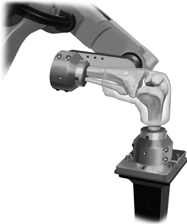
Figure 1. A left knee mounted in an inverted position in the robotic testing device, with the femoral end fixed to a universal force-torque sensor.
